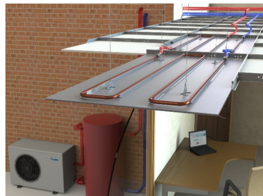
Figure C1.5-1.12 : Radiant ceiling cooling and heating system (S&P,2013)
